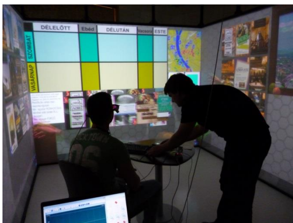
Figure 1: CAVE environment. A triangle shaped desk was placed 230 centimeters from the main wall, in the middle of the space. Participants were seated on the left side of the table.
